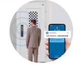
Adopted with the PIR sensor, when someone moves around the front door within 3 meters\*, the AI humanoid detection algorithm will identify abnormal dynamics by instantly capturing a photo or recording a video. Then it will simultaneously push a message to the APP through the encrypted cloud server, which allows you to fully manage the dynamics at the doorway and avoid security risks.
