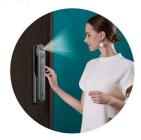
With dual cameras that simulate human eye imaging and obtain 3D features on people's faces, our lock can effectively identify individuals in photos, videos, and even with makeup. The ultrasonic sensor\* initiates facial authentication as you approach within 1 meter of the lock, retracting the latch bolt automatically upon successful recognition. Walk right in without any extra steps!
