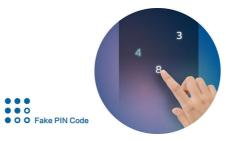
Feature with hidden PIN code technology, Philips smart lock allows you to enter any random number combinations to successfully get identified as long as there is a consecutive input of the real password. This feature can effectively prevent peeping and safeguard your real password.
