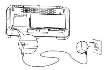
2 Connect the other end of the AC adaptor to the wall outlet.
