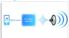
Advanced pure digital sound processing technology offers vastly superior sound performance compared to the conventional analogue audio processing technology that is found in docking players that use the analogue audio output from an iPod/iPhone. By collecting the iPod's/iPhone's digital audio output and employing digital processing at each stage of the circuit, a much higher Signal-to-Noise ratio is produced. The result is unsurpassed sound clarity that is in perfect balance.
