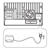
Stick the other end of the GPS antenna to a metal surface of the car.
