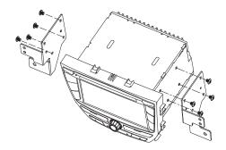
Slide the unit into the dashboard and fix it to the car with four screws.
