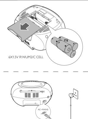
To play with the device, you can use either alkaline battery (R14) or AC power.
