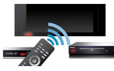
EasyLink lets you control multiple devices like DVD players, Blu-ray players, soundbar speakers, Home theatre systems and TVs etc. with one remote. It uses HDMI CEC industry-standard protocol to share functionality between devices through the HDMI cable. With one touch of a button, you can operate all your connected HDMI CEC-enabled equipment simultaneously. Functions like standby and play can now be carried out with absolute ease.
