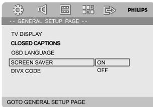
→ **ON**: In STOP, PAUSE or No DISC mode, if no actions are performed about 3 minutes, the screen saver will be activated.
