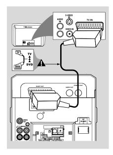
Use the SCART cable (black) to connect the DVD Player's SCART jack (SCART OUT) to the corresponding Scart input jacks on the TV (cable not supplied).
