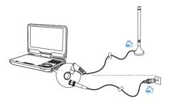
Connect the antenna to the antenna jack.
