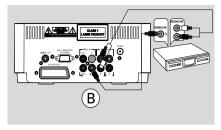
Using the VCR for recording DVDs (B) Connect one of the system's VIDEO OUT jacks to the corresponding VIDEO IN jack and LINE OUT (R/L) jacks to the AUDIO IN jacks on the VCR. This will allow you to make analogue stereo (two channel, right and left) recordings.
