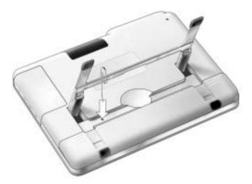
Press the Reset button with a pointed object, such as an unfolded paperclip. The iPronto will reboot. Some settings may be lost, such as date and time settings.
