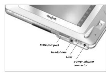
The MMC/SD slot, the headphone connection and the USB port are currently not operational.
