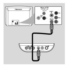
Use a composite video cable (yellow-not supplied) to connect the VIDEO OUT jack on the video box to the video input jack (or labeled as A/V In, CVBS, Composite or Baseband) on the TV.
