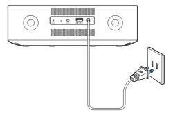
Connect the AC power cord to the wall outlet.
