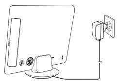
➡ If the PhotoAlbum is powered off, the LED indicators under the left-right slider and the OK button blink during the charging process. When the builtin battery is fully charged, the LED indicators stop blinking.
