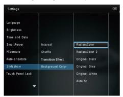
→ If you select [RadiantColor], the PhotoAlbum extends the color on the edges of a photo that is smaller than the full screen to fill the screen without black bars or aspect ratio distortion.
