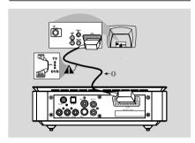
Use the SCART cable (black) to connect the DVD Player's SCART jack (SCART) to the corresponding Scart input jacks on the TV.
