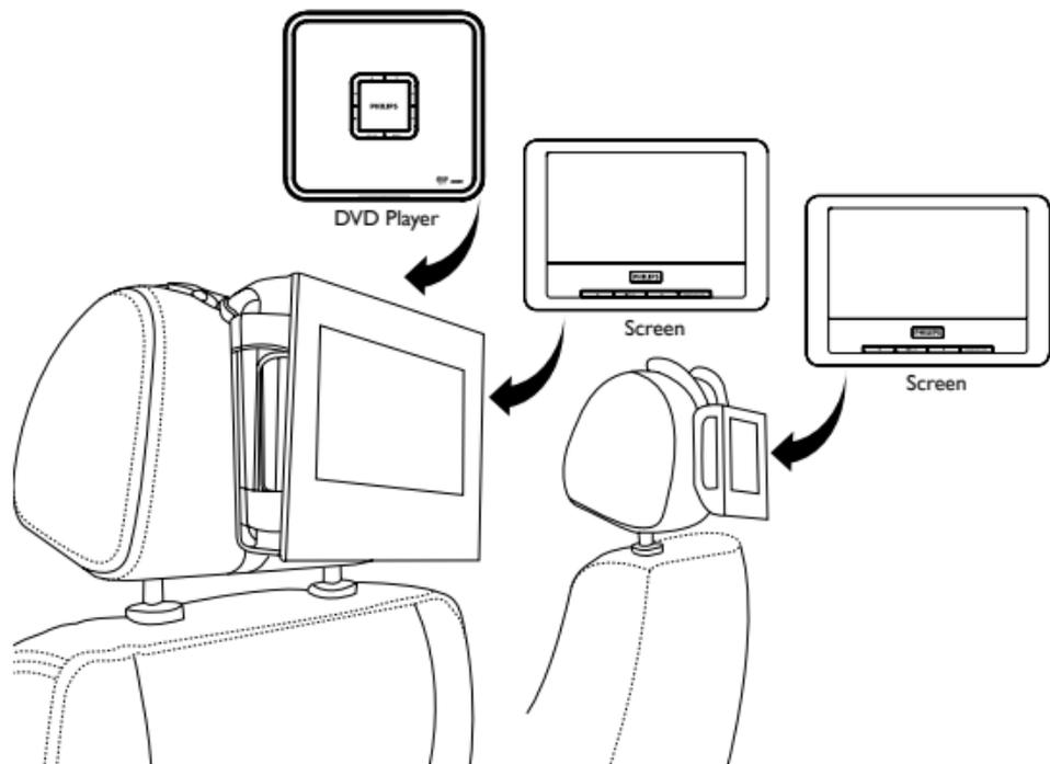
**Tip:** You can place the main DVD player at anywhere in the car as long as the cables length allows. Fasten the pouch straps if you do not put the DVD player inside the pouch.
