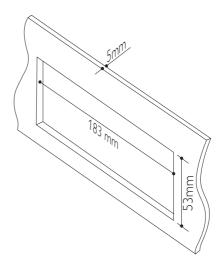
Install the sleeve into the dashboard and bend the tabs outward to fix the sleeve.
