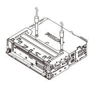
Remove the mounting sleeve with the supplied disassembly tools.
