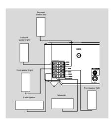
Connect the speaker wires to the SPEAKER terminals by matching the color and silkscreen, coloured (marked) wire to "+" and black (unmarked) wire to "-". Fully insert the stripped portion of the speaker wire into the terminal as shown.
