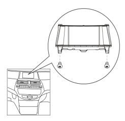
3 Slide the main unit into the car, and fix it to the car with four screws.
