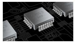
Class D Amplifier takes an analog signal, converts it into a digital signal and then amplifies the signal digitally. The signal then enters a demodulation filter to give the final output. The amplified digital output delivers all the advantages of digital audio, including improved sound quality. In addition, Class 'D' Digital Amplifier has greater than 90% efficiency compared to traditional AB amplifiers. This high efficiency translates into a powerful amplifier with a small footprint.
