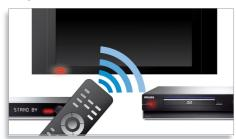
EasyLink lets you control multiple devices with one remote. It uses HDMI CEC industry-standard protocol to share functionality between devices through the HDMI cable. With one touch of a button, you can operate all your connected HDMI CEC enabled equipment simultaneously. Functions like standby and play can now be carried out with absolute ease.
