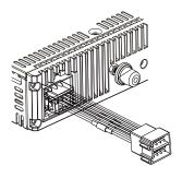
3 Connect the antenna and amplifier as illustrated, if applicable. You can connect the car audio to the amplifier through RCA-TO-RCA cables (not supplied).
