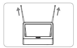
Turn the TV to the desired channel/ station. Move the VHF dipoles in different directions up and down until the reception is achieved.
