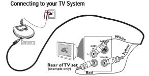
Use the supplied AV cable to connect the player to your TV system. To ensure uninterrupted viewing, we recommend you use AC mains power for your player during VCD operation 1 Insert the yellow video cable pin into the VIDEO IN jack on the rear of your TV.
