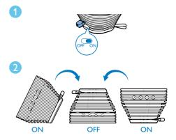
1 Switch the slider to **ON** to enable the auto sensor.
