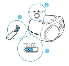
The USB input (as a music source) is meant for data transfer, not for battery charging purpose.
