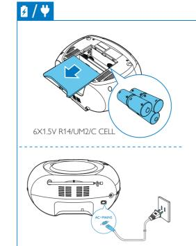
EN To play with the device, you can use either alkaline battery (R14) or AC power.
