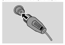
For better FM stereo reception, connect an outdoor FM antenna to the FM AERIAL (FM ANTENNA) terminal.
