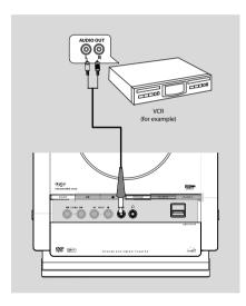
Connect the system's AUX-IN jack to the AUDIO OUT jacks on another audio/visual device (such as a VCR, Laser Disc player or cassette desk) using a "single-to-double" cinch cable (with one end providing a 3.5" connector for connection to the AUX-IN jack while the other end providing two white/red connectors for connection to the other device's AUDIO OUT jacks).
