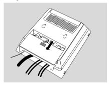
② Align the side marked **PRESS** ▼ of the stand to the slots at the bottom of the set.
