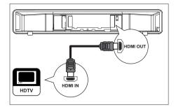
Connect a HDMI cable (supplied) from the HDMI OUT on this unit to the HDMI IN socket on your TV.
