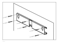
7 Hook the DVD Home Theatre unit firmly onto the mounted bracket. Slide the knobs through the key holes and lock into position.
