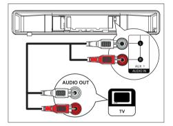
1 Connect an audio cable (not supplied) from the AUDIO IN-AUX1 sockets on this unit to the AUDIO OUT sockets on your TV.
