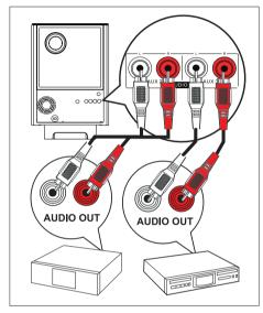
1 Connect an audio cable (not supplied) from the AUDIO IN-AUX2 or AUX3 sockets on the subwoofer to the AUDIO OUT sockets on the device.
