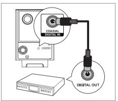
1 Connect a coaxial cable (not supplied) from the DIGITAL IN-COAXIAL socket on the subwoofer to the COAXIAL/ DIGITAL OUT socket on the device.
