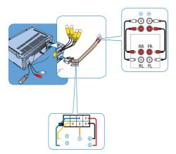
Illumination switch To the +12V car battery which is energized at all time Motor/electric antenna relay control lead/ Amplifier relay control lead Ground Ignition Key +12V DC when ON/ **ACC** Antenna Aux-In Parking Switch Cable Reverse Driving Cable (10)Video-In <u>(11)</u> Camera-In Video-Out 1 and 2 Rear line-Out Front line-Out
