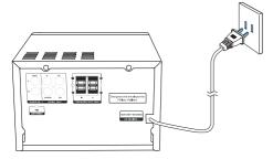
Connect the AC power cord to the wall power socket.
