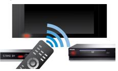
EasyLink lets you control multiple devices like DVD players, Blu-ray players, soundbar speakers, Home theatre systems and TVs etc. with one remote. It uses HDMI CEC industrystandard protocol to share functionality between devices through the HDMI cable. With one touch of a button, you can operate all your connected HDMI CEC-enabled equipment simultaneously. Functions like standby and play can now be carried out with absolute ease.
