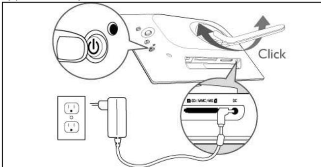
**Note:** For safety reason and best stability Philips recommend to adjust the stand with the angle defined by the two clicked position. Using other positions may cause the PhotoFrame™ to fall and is under the entire responsibility of the user.
