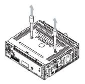
4 Remove the mounting sleeve with the supplied disassembly tools.
