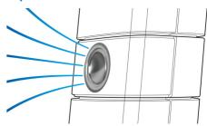
Unique speakers designed with exposed tweeters to give maximum dispersion and openness in the sound.
