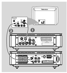
Use an S-Video cable (not supplied) to connect the DVD system's S-VIDEO jack to the S-Video input jack (or labeled as Y/C or S-VHS) on the TV.
