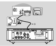
Use the SCART cable (black) to connect the DVD Player's SCART jack (SCART) to the corresponding Scart input jacks on the TV.
