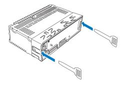
Install the sleeve into the dashboard and bend the tabs outward to fix the sleeve.
