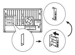
If the fuse gets damaged immediately after it has been replaced, there may be an internal malfunction. In such case, consult your Philips dealer:
