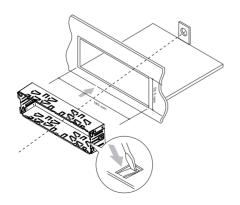
Place the supplied rubber cushion over the end of the mounting bolt.
