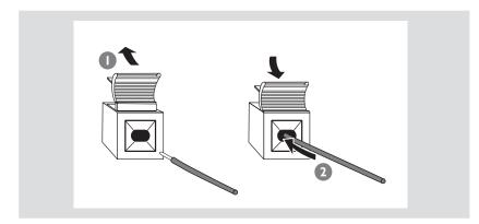
Fully insert the stripped portion of the speaker wire into the terminal as shown.
