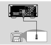
Use a HDMI cable (not supplied) to connect the HDMI jack on the DVD Player to HDMI IN on a HDMI compatible device (e.g.; TV, Projector; Adaptor).
