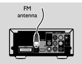
Connect the supplied FM antenna to the FM ANENNA (75 Ω) jack. Extend the FM antenna and fix its end to the wall. For better FM stereo reception, connect an
