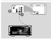
Use the supplied composite video cable (yellow) to connect the DVD system's VIDEO jack to the video input jack (or labeled as A/V In, CVBS, Composite or Baseband) on the TV.
