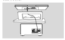
Connect the subwoofer to the main unit with the supplied system cable (grey).
