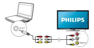
Match the color of the AV cables (the AV cable connected to TV is not supplied) with the jacks:
