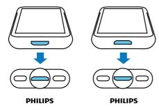
**3** Adjust the bumpers on both sides of the connector to stabilize the phone.
