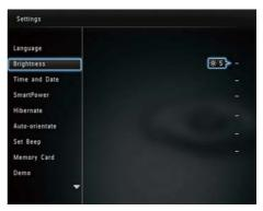
3 Move the joystick up/down to adjust brightness, and then press OK.
