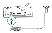
2 Connect the power cord to a power supply socket.
