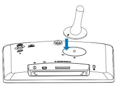
2 Turn the stand anti-clockwise 45 degrees to the <sup>a</sup> position and lock it to the PhotoFrame firmly.
