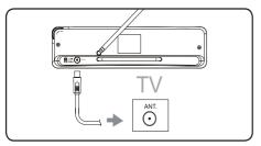
3 Connect the DC plug to the antenna and the power supply to a 100-240V AC outlet.
