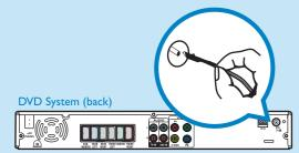
2 Unfold the AM/ MW loop antenna and fix the claw into the slot.
