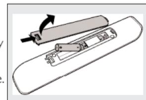
*Note: If the device indicators in the selector window (DVD, STB, VCR, CD and AMP) and the Standby key blink four times after every key press, the remote control is indicating that its batteries are running low. Replace the old batteries with two new AAA batteries.*
