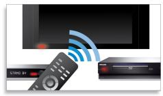
EasyLink lets you control multiple devices like DVD players, Blu-ray players, TV's etc. with one remote. It uses HDMI CEC industry-standard protocol to share functionality between devices through the HDMI cable. With one touch of a button, you can operate all your connected HDMI CEC enabled equipment simultaneously. Functions like standby and play can now be carried out with absolute ease.
